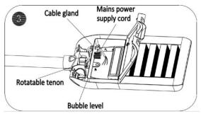
**STEP 4:** Get mains power supply cord into led driver compartment via cable gland, and use open spanner or similar tool to lock the gland to mains power supply cord tightly. **See Figure 3.**
